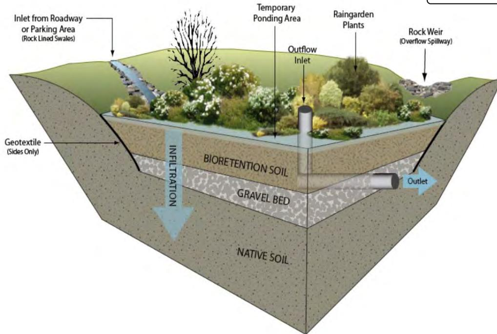
Image 2-3 is a cross section schematic of a bioretention cell. Bioretention cells are shallow landscaped depressions that incorporate plantings and engineered soil with a high porosity and infiltration capacity. Bioretention cells control stormwater runoff volume by providing storage, reducing peak discharge, and removing pollutants through physical, chemical, and biological processes occurring in plants and soil.
